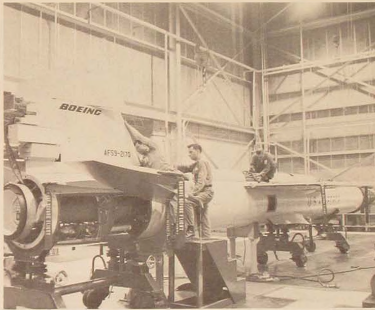
Inspection of the pressure system valves and of the tail section installation.
