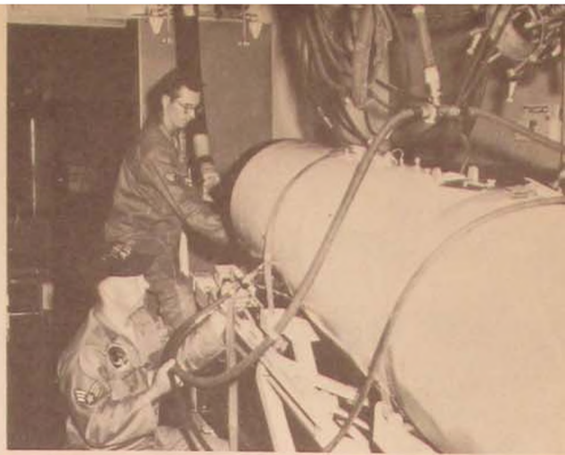
Bomarc maintenance technicians hook up a ramjet engine for testing in the Hurlburt assembly and maintenance building.
