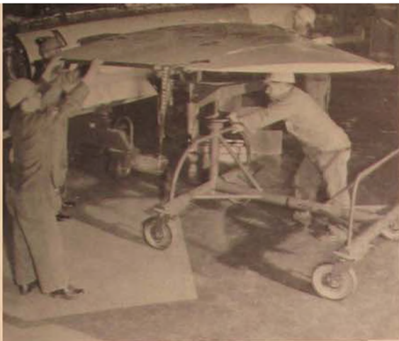
Technicians use special mobile equipment to align and install a wing section.
