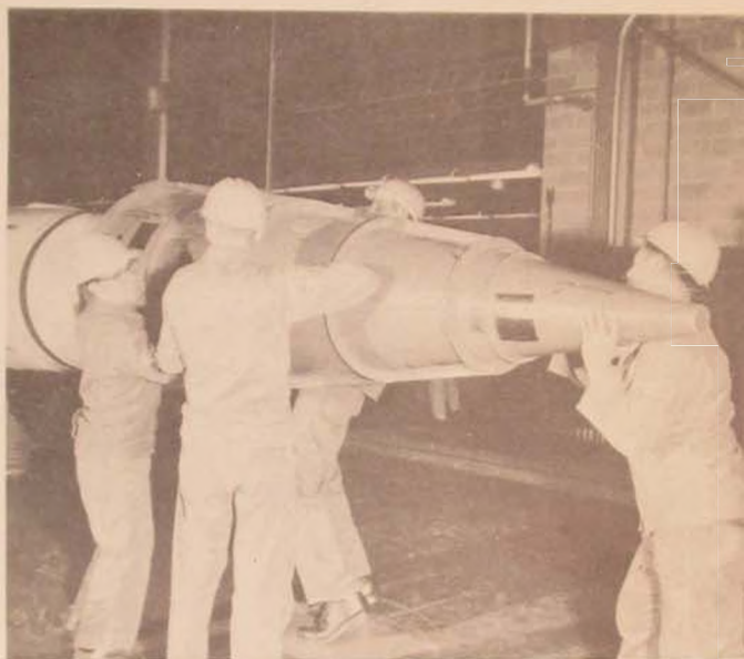
Removing the protective casing from the pointed fiberglass radome nose cone.
